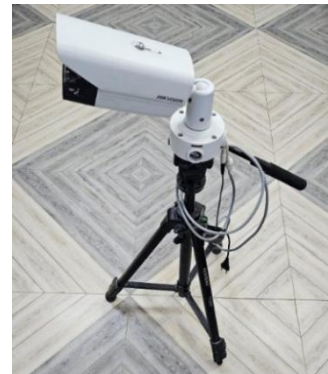
Fig. 2. Thermal camera mounted on tripod for stable video capture.
