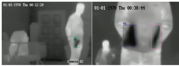
Fig. 6. Tracking gun and knife across frames using GNN, with unique IDs and bounding boxes.
