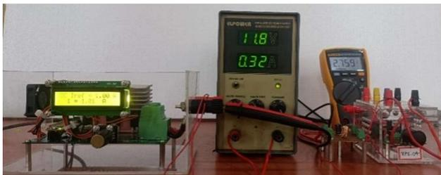
Fig. 10. Experimental set-up to validate DC-DC buck converter.
