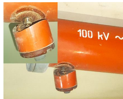
Fig. 9. Misconnection issue in the measuring capacitor.
