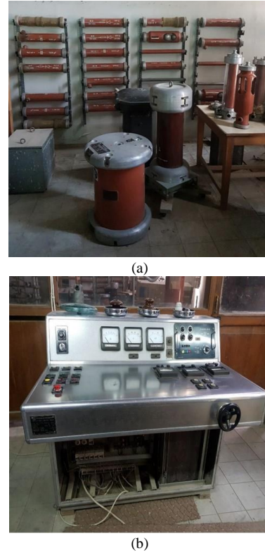
Fig. 1. Bamberg kit: (a) Components and (b) Control desk.
