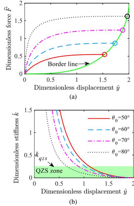
Fig. 2. The dimensionless force and stiffness versus displacement of proposed model with different initial angel. (a) Dimensionless force  $\hat{F}$ ; (b) Dimensionless stiffness  $\hat{k}$ . “Solid line —” for  $\theta_0 = 50^\circ, \alpha = 0.36$ ; “Dash line - -” for  $\theta_0 = 60^\circ, \alpha = 0.5$ ; “Dash dot line - · -” for  $\theta_0 = 70^\circ, \alpha = 0.66$ ; “Dot line ...” for  $\theta_0 = 80^\circ, \alpha = 0.83$ .
