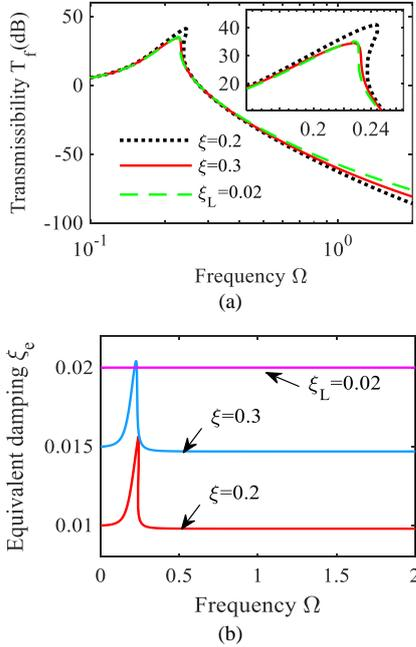
Fig. 5. Force transmissibility and equivalent damping ratio of the system under different damping coefficients for  $\theta_0 = 60^\circ, \alpha = 0.5, f_0 = 0.002$ . (a) Force transmissibility; (b) equivalent damping ratio.
