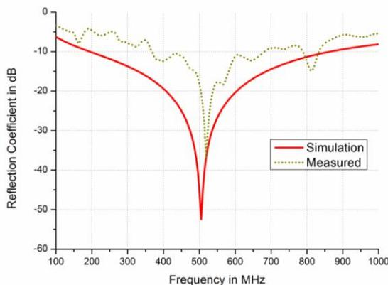
Fig. 8. Simulated and measured reflection coefficient.
