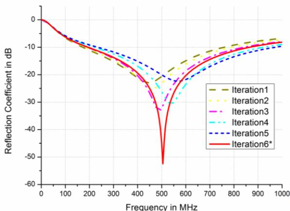
Fig. 4. The reflection coefficient for various ground plane height.
