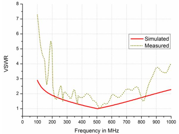
Fig. 9. Simulated and measured VSWR.
