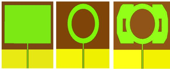
Fig. 2. Configuration of various steps involved in the designed antenna.
