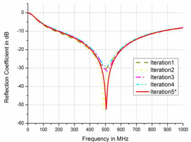
Fig. 5. The reflection coefficient for various feed line width.
