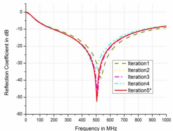
Fig. 6. The reflection coefficient for various circular radiuses.
