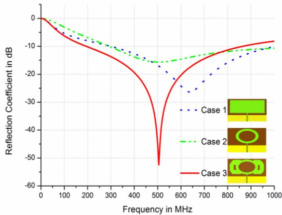
Fig. 3. The reflection coefficient of steps involved in the design.
