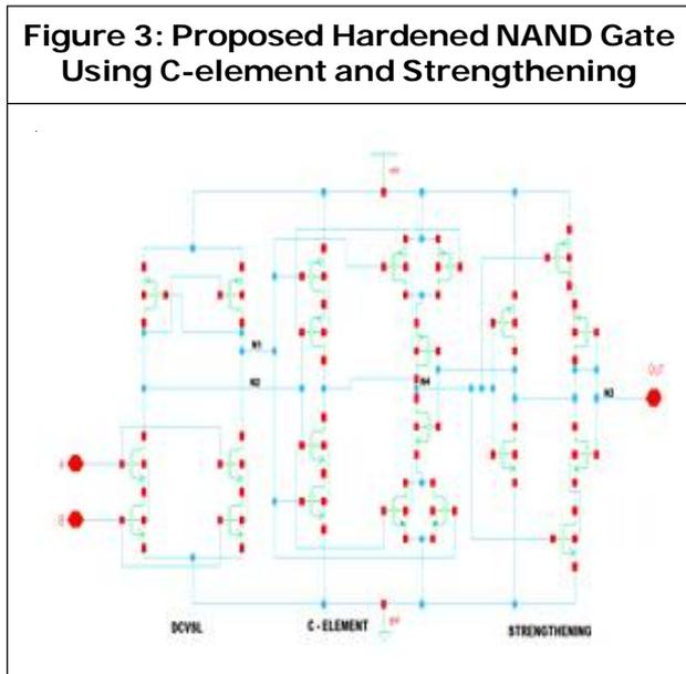
style fashion and thus combine differential logic and positive feedback. As a result both the output nodes provide the same logic function OUT\_BAR.
