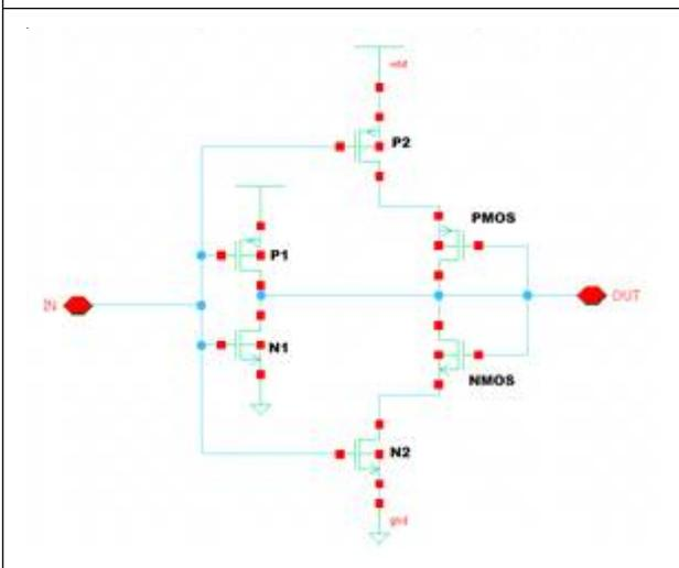
memory element. The concept of strengthening (Calomarde *et al.*, 2013) is to make the logic gates more robust to the SET at the sensitive nodes.
