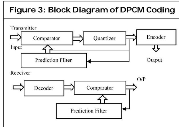
Since the difference between input samples is less than a whole input sample, the number of bits required for transmission is reduced (Yadav Monika S *et al.*, 2016). DPCM quantizes the difference signal using uniform quantization. Uniform quantization produces an SNR that is slight for small input sample signals and large for huge input sample signals. Hence, voice quality is well at higher signals.
