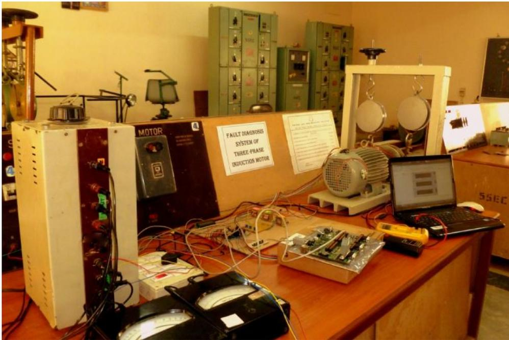
50 Hz coupled to a mechanical load. One motor is healthy and the observations were considered as reference to compare with the other motor which has a bearing fault.
