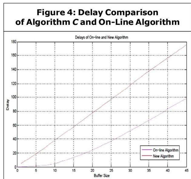
of a small increase in the overall delay of the system. It can be seen from the above Figure 4, the delay of Algorithm C is more than delay of On-line algorithm thus giving out a better rate jitter which is the main interest of this thesis.
