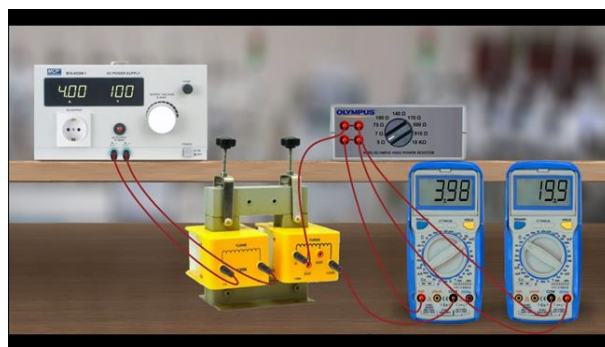
Fig. 1. Screenshot from the EVEEE environment, presenting a VL for investigation of a laboratory transformer
