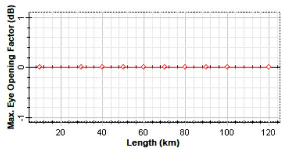
Fig. 14. EOP vs Fiber Length for the 256-QAM modulation scheme.
