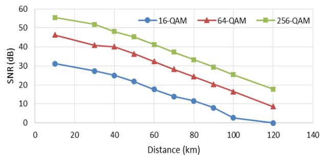
Fig. 9. SNR vs transmission distance at 5Gbps data rate for three different modulation schemes.
