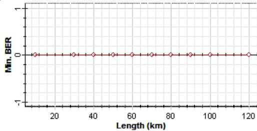
Fig. 6. BER for 256-QAM modulation scheme.
