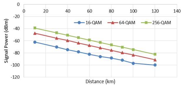
Fig. 7. Received power vs transmission distance at 5Gbps data rate for three different modulation schemes.
