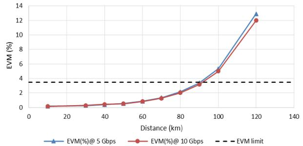
Fig. 13. EVM vs Fiber Length for the 256-QAM modulation scheme.
