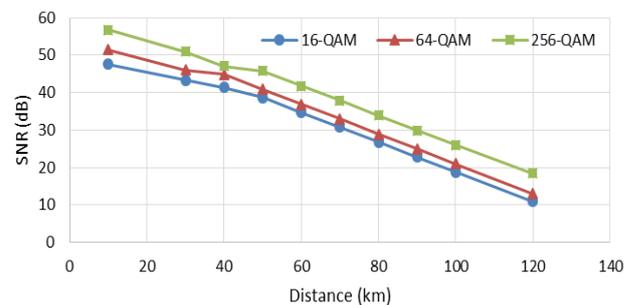
Fig. 10. SNR vs transmission distance at 10Gbps data rate for three different modulation schemes.
