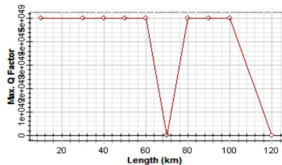
Fig. 5. Q-factor for 256-QAM modulation scheme.
