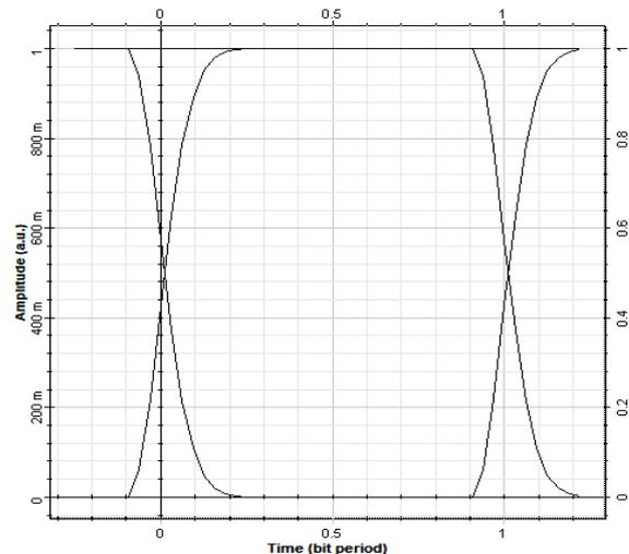
Fig. 15. Eye diagram for the 256-QAM modulation scheme.
