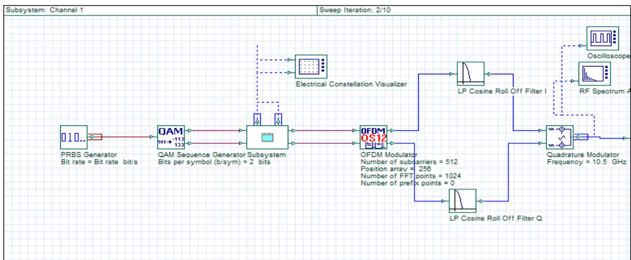
Fig. 2. RF transmitter of the SCM-OFDM channel 1.
