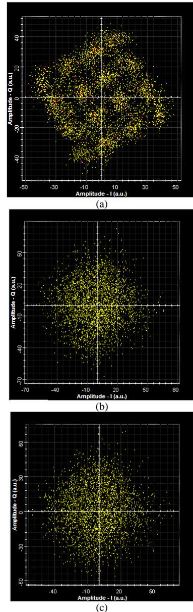
Fig. 16. SCM-OFDM RoF system constellation diagram at 90 km for 10 Gbps data rate, (a) 16-QAM, (b) 64-QAM and (c) 256-QAM.
