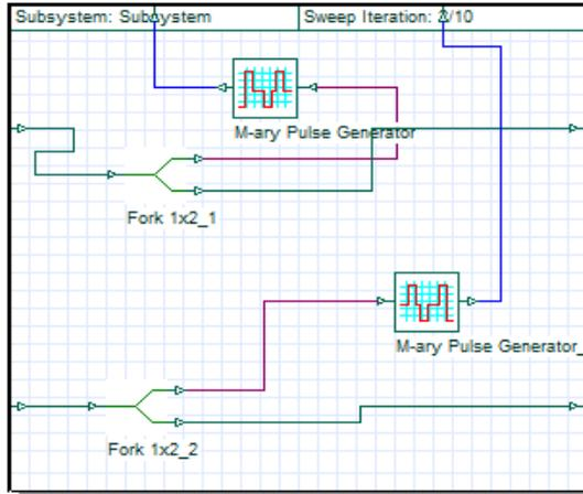
Fig. 3. M-ary pulse generator subsystem.
