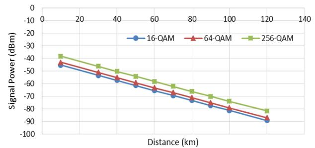
Fig. 8. Received power vs transmission distance at 10Gbps data rate for three different modulation schemes.
