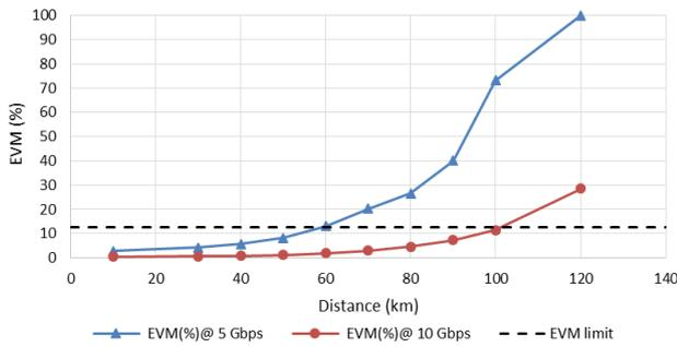
Fig. 11. EVM vs fiber length for the 16-QAM modulation scheme.
