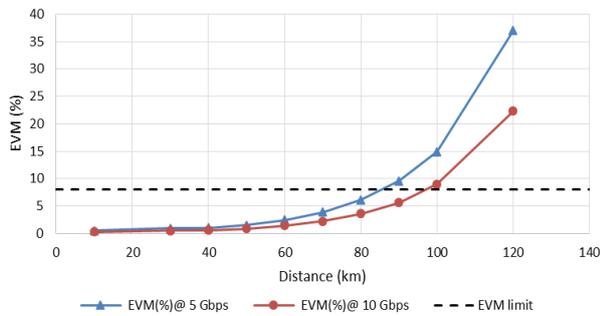
Fig. 12. EVM vs fiber length for the 64-QAM modulation scheme.
