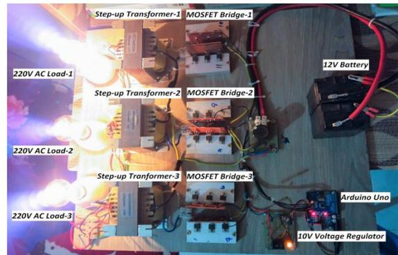
Fig. 15. Practical implementation of the designed three-phase inverter in its ON condition.
