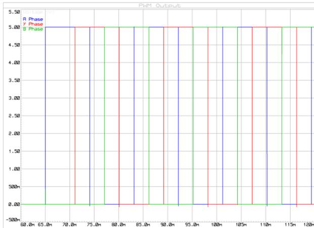
Fig. 8. PWM voltages from Arduino with 120° phase displacement.
