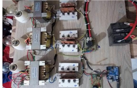
Fig. 14. Practical setup of the designed three-phase inverter.
