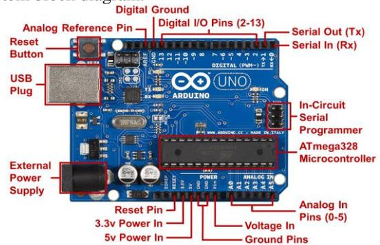
Fig. 3. Arduino Uno R3 with pin-outs.
