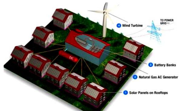
Fig. 1. A typical microgrid system [7], [8].
