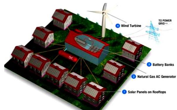
Fig. 1. A typical microgrid system [7], [8].
