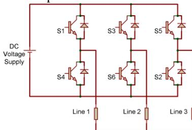
Fig. 2. A basic voltage source three-phase Inverter [9].
