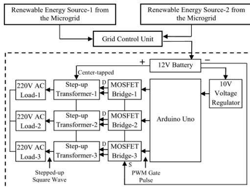
Fig. 5. Block diagram of the designed three-phase inverter system.
