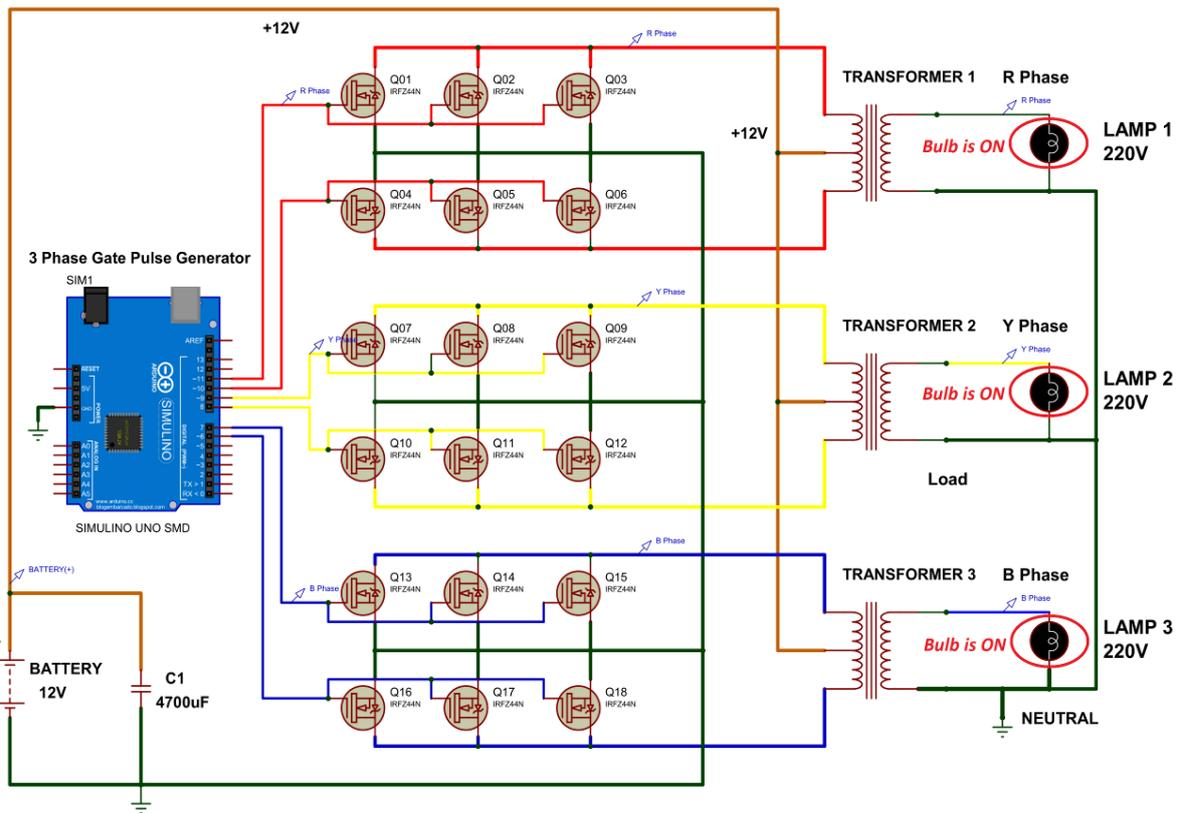
Fig. 7. Operational simulation result of the three-phase inverter.
