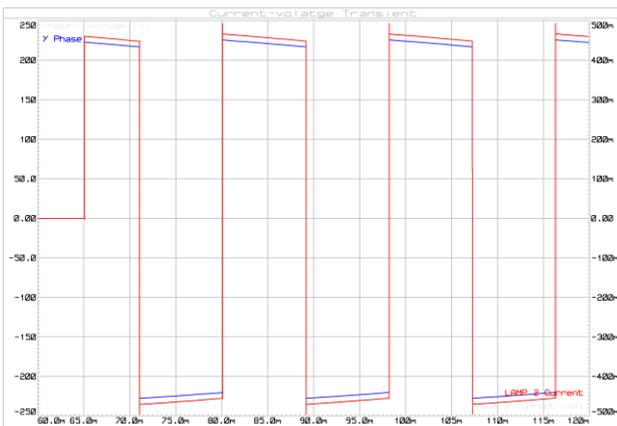
Fig. 12. Voltage vs current transient response at Phase-Y.
