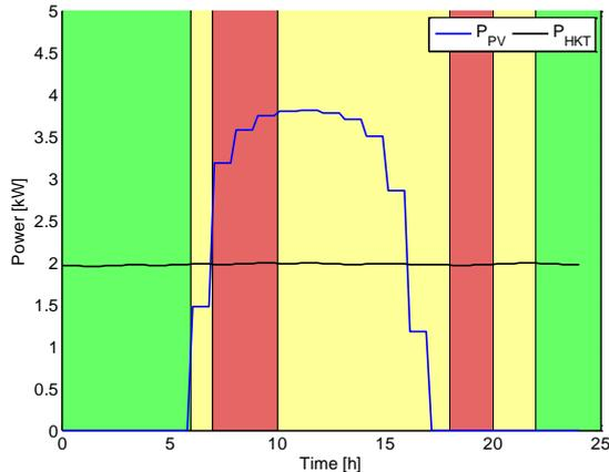
Fig. 3. Photovoltaic and hydrokinetic systems' output power.
