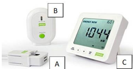
Fig. 3. Eferyg wireless electricity monitor and data logger.
