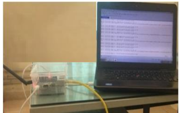
Fig. 11. Gateway placed inside a room for reception across concrete obstructions.
