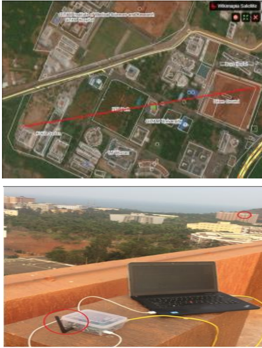
Fig. 9. (Top) Map of the field trial location. (Bottom) The red circles mark the locations of receiving third party whip antenna (lower left) and transmitting PCB antenna (upper right). The transmission takes place in free space along the line of sight marked by the red line in the map.
