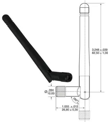
Fig. 8. Dimensions of the third party whip antenna.
