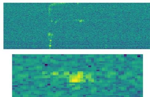
Fig. 5. Raw data (top) and ROI data (bottom): both first cyclist data with ID=1.
