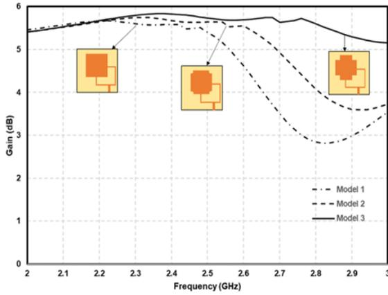
Fig. 5. Comparison of gain of the development model.
