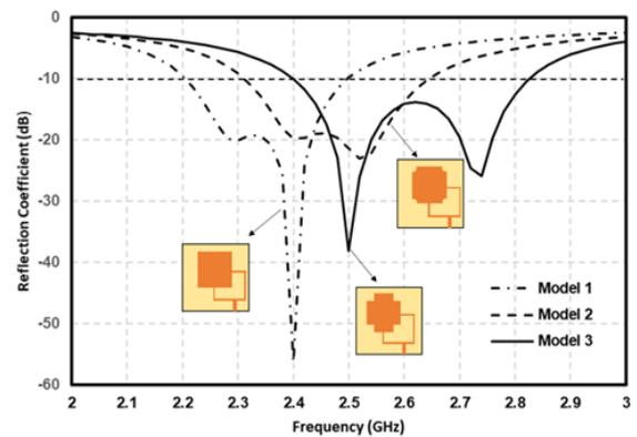
Fig. 3. Comparison of the reflection coefficient of the development model.
