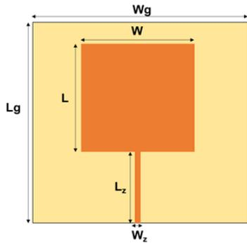
Fig. 1. Design of square patch microstrip antenna.
