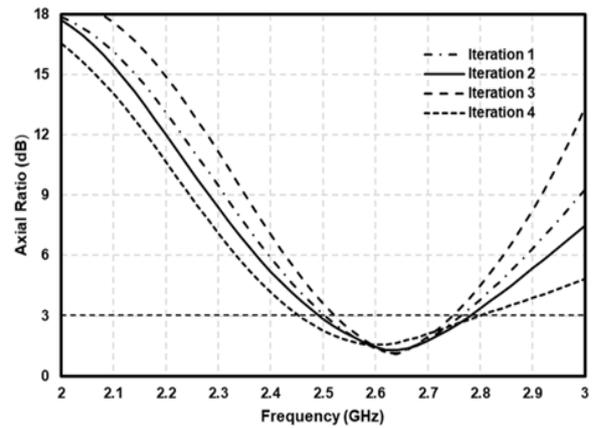
Fig. 7. Simulation of axial ratio from Iteration of  $L_4$ .
