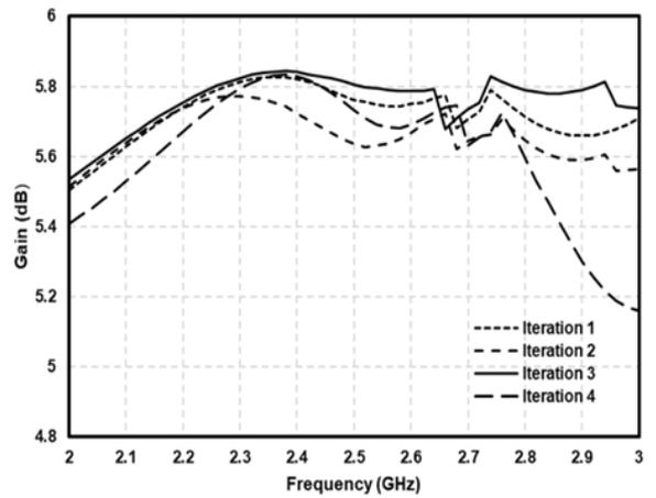
Fig. 8. Simulation of gain from Iteration of  $L_4$ .
