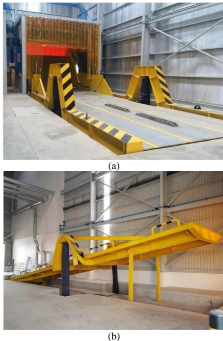
Fig. 4. Illustration of the truck dumper: (a) machine in the idle stage, and (b) machine in the working stage (Photos courtesy: Kasetphand Industry Co., Ltd., Thailand)
