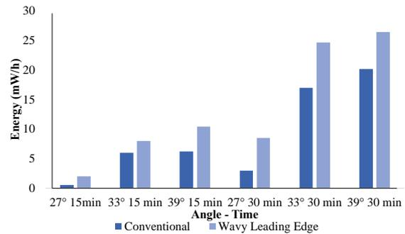
Fig. 7. Energy measurements for both turbines at different angles of attack.
