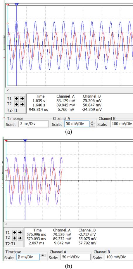
Fig. 10. Output waveform with the load for (a) SG MOSFET and (b) DG MOSFET based class-AB amplifier.
