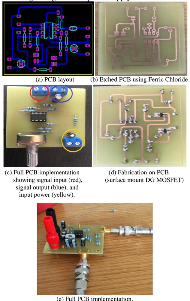
Fig. 11. Fabrication process of the DG MOSFET based class-AB amplifier.
