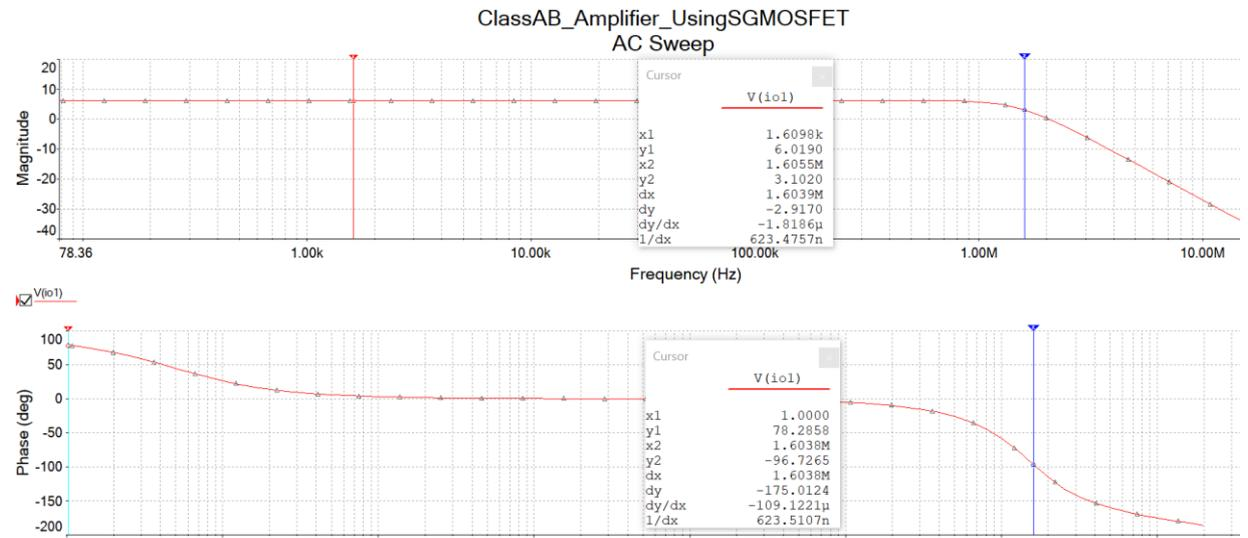
(c) Higher cut-off frequency for SG MOSFET based class-AB amplifier
