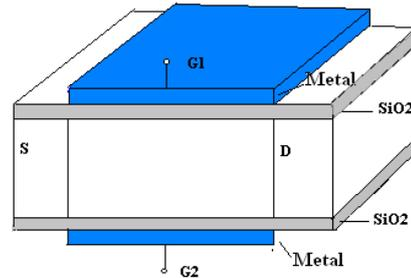
Fig. 2. Schematic of the DG MOSFET [25]. (S: Source, D: Drain, G<sub>1</sub> and G<sub>2</sub>: Gate-1 and gate-2, SiO<sub>2</sub>: Silicon di-oxide)
