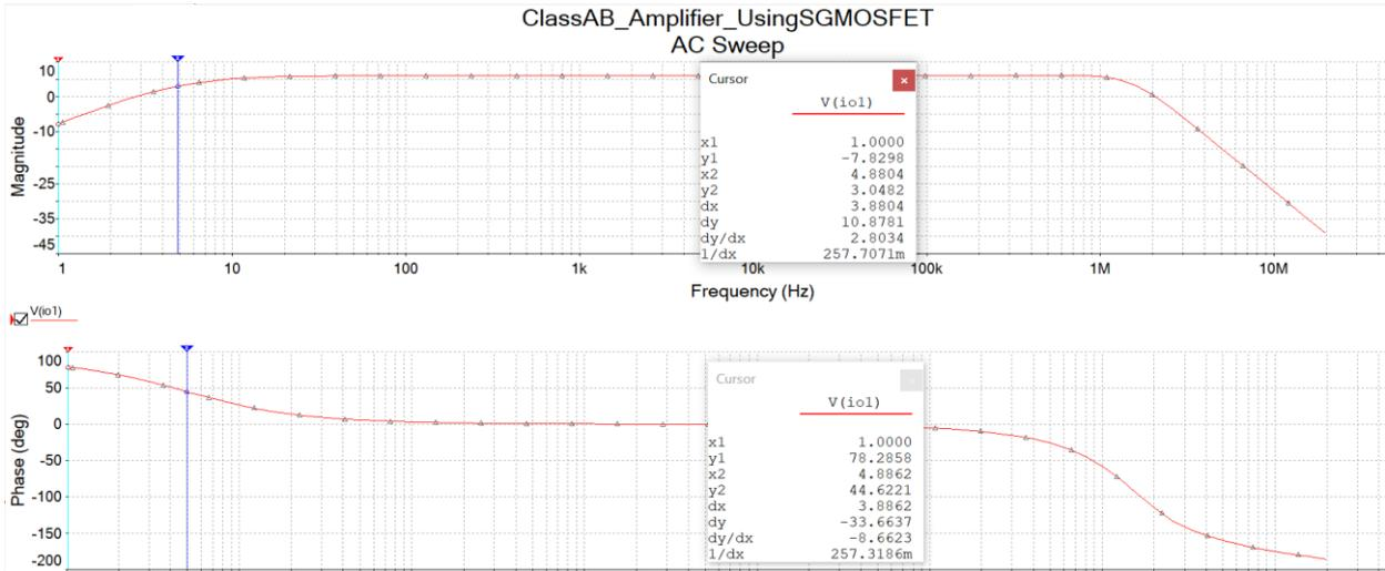
(a) Lower cut-off frequency for SG MOSFET based class-AB amplifier
