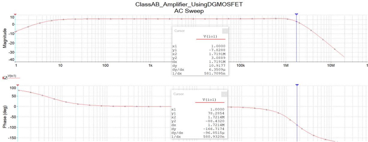
(d) Higher cut-off frequency for DG MOSFET based class-AB amplifier
