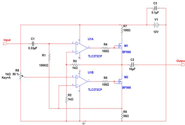
Fig. 6. Complete circuit design of class-AB amplifier using DG MOSFET.
