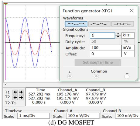
Fig. 9. Gain preservation at  $V_{cc} = 6.5$  V for the designed class-AB amplifier circuit at 10 mVpk signal (a) and (b), and at 100 mVpk signal (c) and (d).
