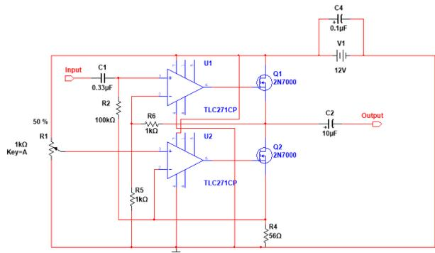
Fig. 5. Circuit design of class-AB amplifier using SG MOSFET.
