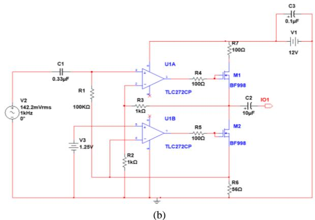
Fig. 7. (a) SG MOSFET and (b) DG MOSFET based class-AB amplifier with AC input signal.
