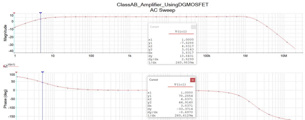
(b) Lower cut-off frequency for DG MOSFET based class-AB amplifier
