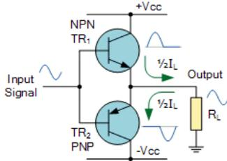
Fig. 4. Basic topology of class-AB amplifier [30].
