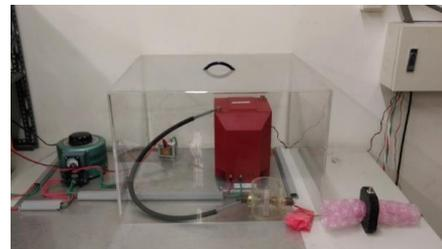
Fig. 1. High-voltage PD simulation platform.
