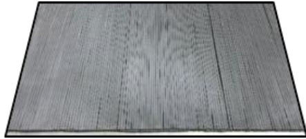
Fig. 3. Design 1: Carbon coated microwave absorber.
