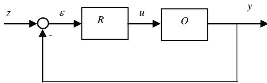
Fig. 1. A closed loop control system.
