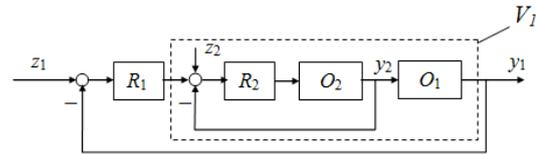
Fig. 7. Two-loops control system and equivalent single-loop structure to  $R_1$  controller.
