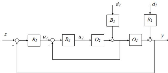
Fig. 4. Block diagram of cascade control system.
