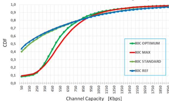
Fig. 7. CDF for the two proposed channel assignment mechanisms with 80 sensor pairs and a threshold  $CC_{th} = 250$  Kbps.
