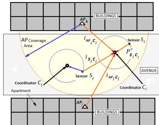
Fig. 2. Interference on a coordinator sensor pair.
