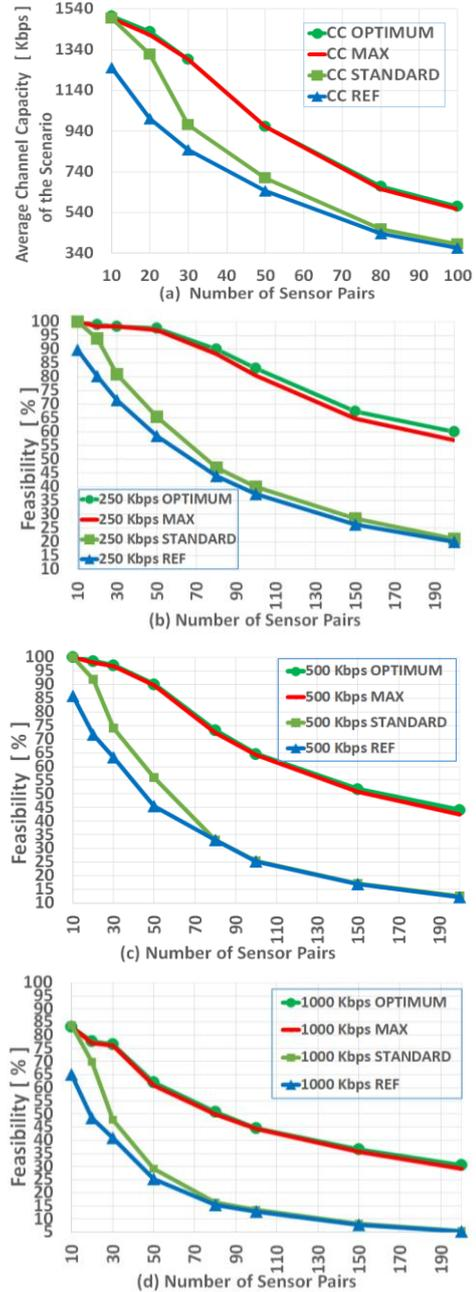
Fig. 6. (a) Average channel capacity for the two channel assignment mechanisms plus standard channel assignment method and reference REF vs number of sensor pairs, (b) feasibility for the two channel assignments mechanisms with a threshold of  $CC_{th} = 250$  Kbps, (c) feasibility for the two channel assignments mechanisms with a threshold of  $CC_{th} = 500$  Kbps, and (d) feasibility for the two channel assignments mechanisms with a threshold of  $CC_{th} = 1000$  Kbps.
