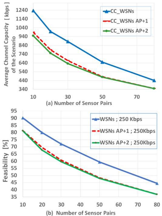
Fig. 3. The performance of WSN vs number of sensor pairs: (a) Channel capacity for different levels of interference and (b) feasibility for  $CC_{th}=250$  Kbps.
