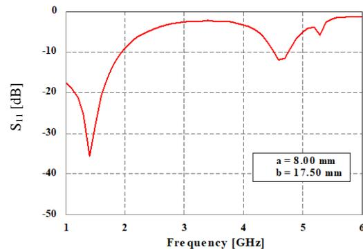
Fig. 2. Return loss of the antenna using the inner radius ( $a = 8$  mm.) and outer radius ( $b = 17.5$  mm.) as calculated from antenna design.
