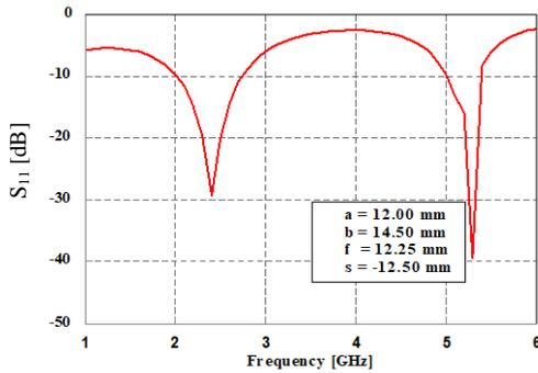
Fig. 8. Simulated result for the dual-band of the microstrip antenna.
