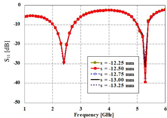
Fig. 7. Return loss of different short-pin positions (the inner radius =  $12.00$  mm, the outer radius =  $14.50$  mm and the feed point =  $12.50$  mm).
