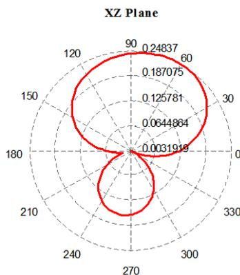
Fig. 9. Directional radiation pattern of 2.4 GHz in the XZ plane.
