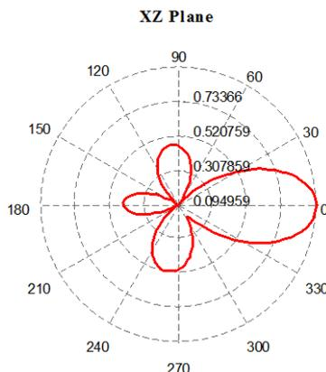
Fig. 10. Directional radiation pattern of 5.3 GHz in the XZ plane.
