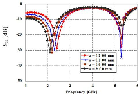
Fig. 4. Return loss of each inner radius (the outer radius =  $14.5$  mm, the feed point =  $12.75$  mm, the short-pin position =  $-12.75$  mm).
