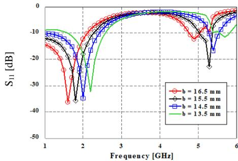
Fig. 3. Return loss of each outer radius (the inner radius =  $8$  mm, the feed point =  $12.75$  mm, the short-pin position =  $-12.75$  mm).
