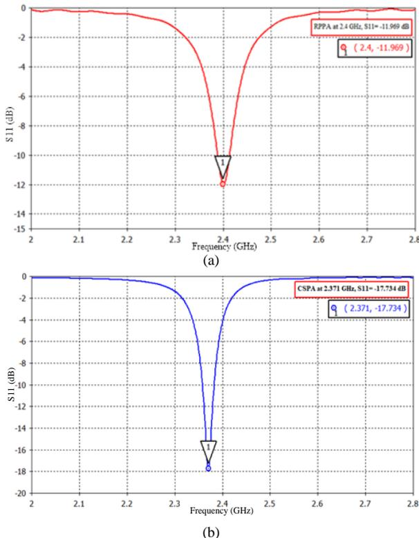
Fig. 4. Return loss of (a) rectangular planar patch antenna and (b) cylindrical surrounding patch antenna.
