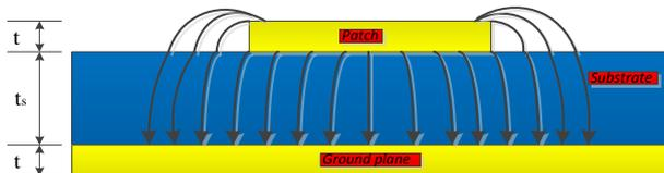
Fig. 3. Electric field lines.
