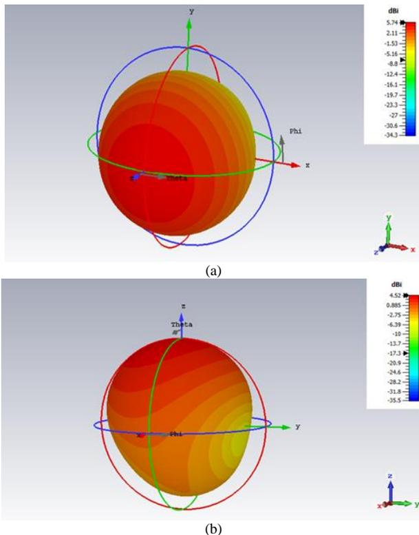
Fig. 6. Gain of (a) rectangular planar patch antenna and (b) cylindrical surrounding patch antenna.
