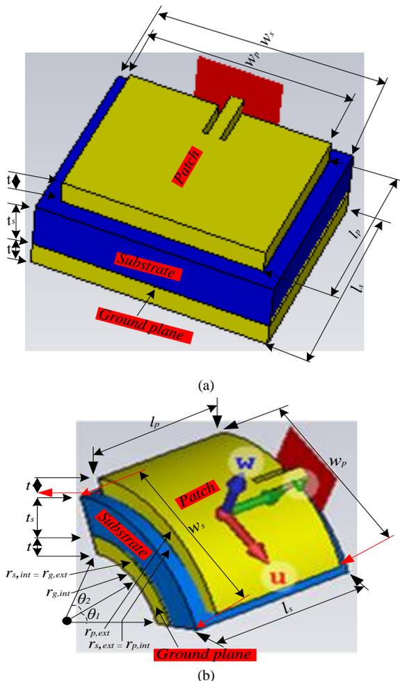
Fig. 1. Parameters observation for (a) planar patch and (b) designed circular patch.
