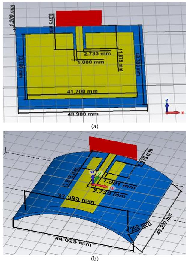
Fig. 2. Geometry of (a) rectangular planar patch antenna (RPPA) and (b) cylindrical surrounding patch antenna (CSPA).
