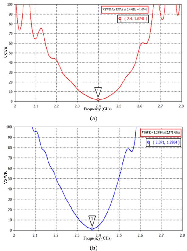
Fig. 5. Voltage standing wave ratio of (a) rectangular planar patch antenna and (b) cylindrical surrounding patch antenna.
