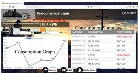
Fig. 8. Consumption monitor page of the enermon.tech user Interface
