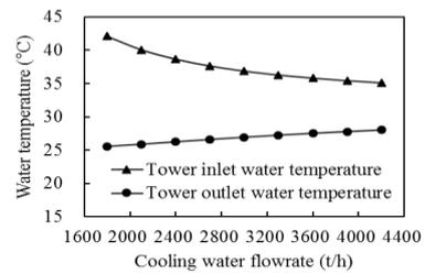
Fig. 4. Influence of cooling water flowrate on the tower inlet and outlet water temperature.
