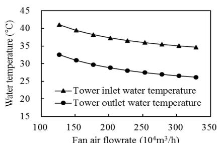
Fig. 8. Influence of fan air flowrate on the tower inlet and outlet water temperature.
