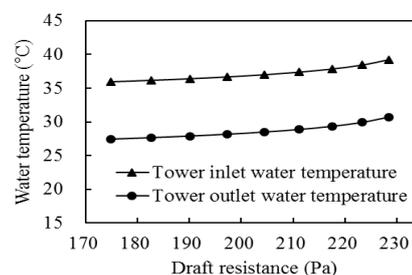
Fig. 7. Influence of draft resistance on the tower inlet and outlet water temperature.
