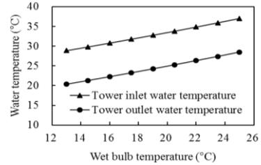
Fig. 3. Influence of wet bulb temperature on the tower inlet and outlet water temperature.
