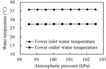
Fig. 1. Influence of atmospheric pressure on the tower inlet and outlet water temperature.
