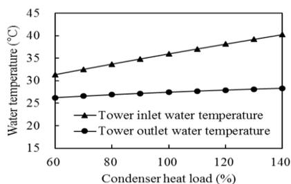
Fig. 5. Influence of condenser heat load on the tower inlet and outlet water temperature.
