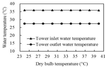
Fig. 2. Influence of dry bulb temperature on the tower inlet and outlet water temperature.
