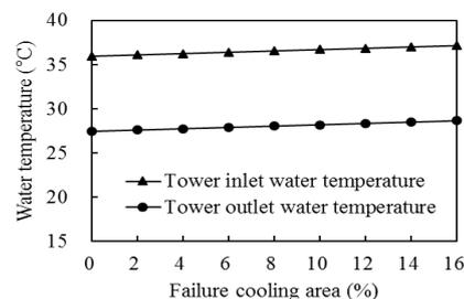
Fig. 6. Influence of failure cooling area on the tower inlet and outlet water temperature.
