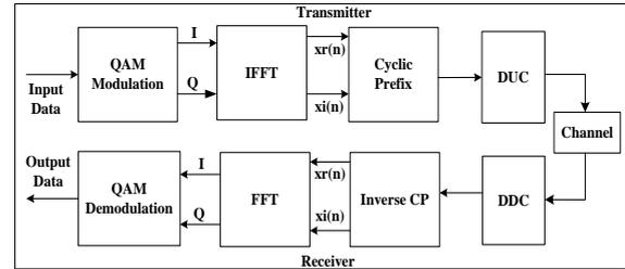
Fig. 4. Proposed RF OFDM block diagram.
