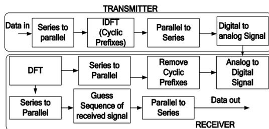
Fig. 1. Transmitter and receiver of OFDM.
