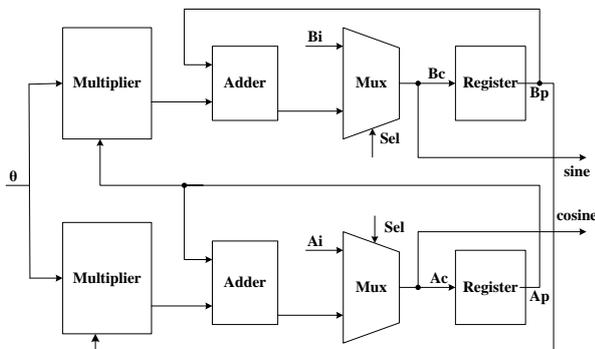
Fig. 3. The hardware architecture of DFS.
