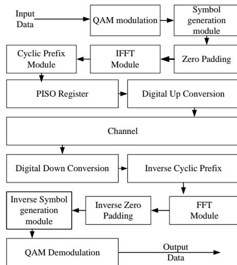
Fig. 2. The architecture of proposed DUC/DDC based OFDM system.
