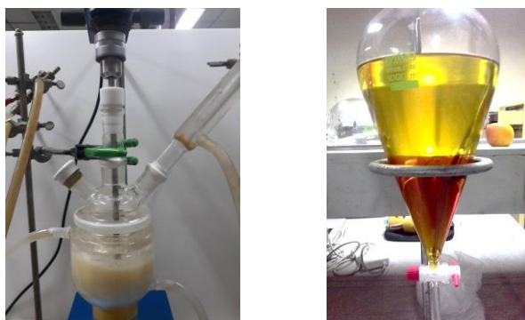
(a) Reaction process (b) Separation between EE and glycerin
