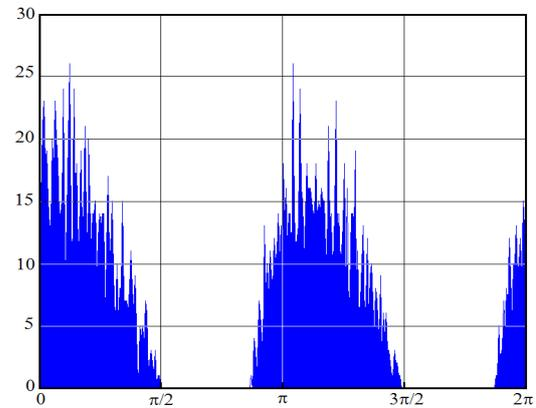
Fig. 3. Example of the 2-d PD current pulses pattern.
