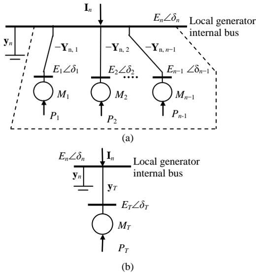
Fig. 2. Equivalent systems: (a) Equivalent of remaining system  $D$  as seen by the local generator and (b) single-generator dynamic equivalent of remaining system  $D$
