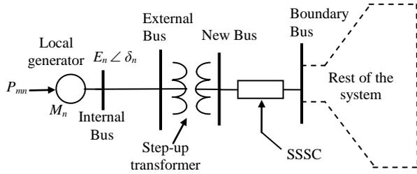
Fig. 4. Power System at the site of  $n$ th local generator with SSSC connected.
