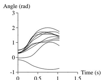
Fig. 12. SBS trajectories for fault case 8 at FCT of 0.28 s with local controls applied.
