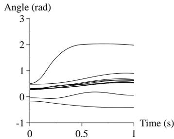
Fig. 5. SBS trajectories for fault case 1 at FCT of 0.15 s with local controls applied.
