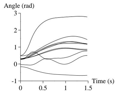
Fig. 9. SBS trajectories for fault case 5 at FCT of 0.20 s with local controls applied.
