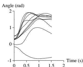
Fig. 10. SBS trajectories for fault case 6 at FCT of 0.26 s with local controls applied.
