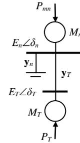
Fig. 3. Localized power system (LPS) model at the site of  $n$ th generator.
