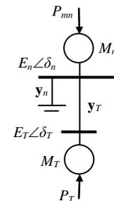
Fig. 3. Localized power system (LPS) model at the site of  $n$ th generator.
