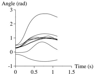
Fig. 8. SBS trajectories for fault case 4 at FCT of 0.27 s with local controls applied.
