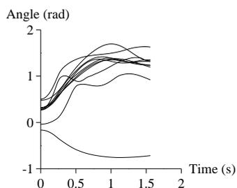
Fig. 11. SBS trajectories for fault case 7 at FCT of 0.21 s with local controls applied.
