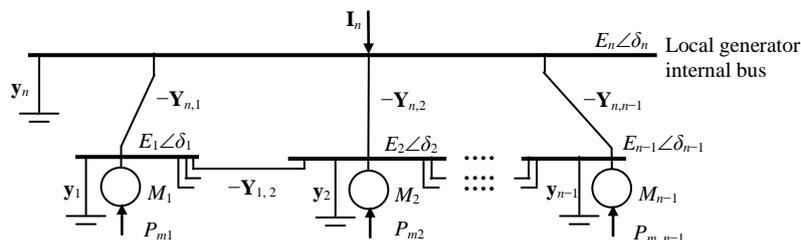
Fig. 1. Remaining system  $D$  (the power system external to the local generator internal bus)
