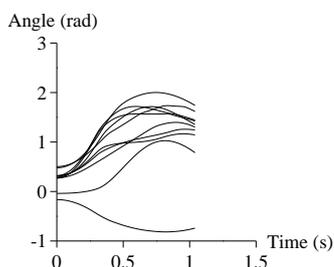
Fig. 12. SBS trajectories for fault case 8 at FCT of 0.28 s with local controls applied.
