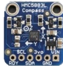
Figure 6. A 3-Axis Magnetometer Sensor (Source: Adafruit Industries, 2017)
