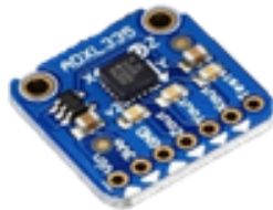
Figure 4. A 3-Axis Accelerometer Sensor (Source: Adafruit Industries, 2017)
