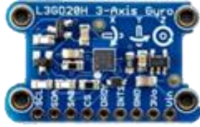
Figure 3. A 3-Axis Gyro Sensor (Source: Adafruit Industries, 2017)
