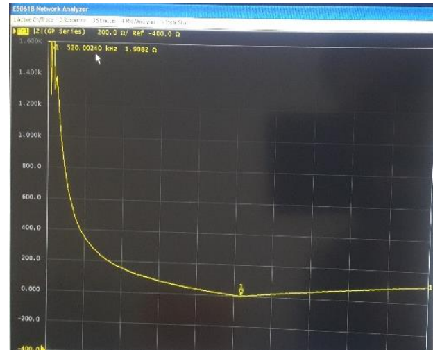
Figure 4. Frequency response of Class-E inverter prototype.
