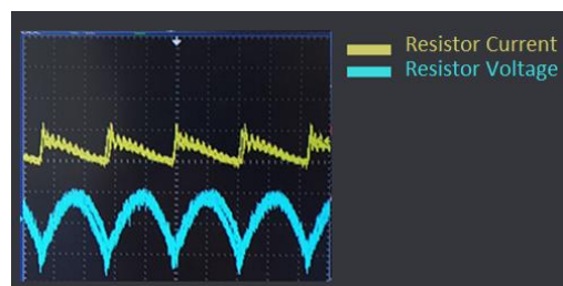
Figure 8. Load voltage and current waveforms with rectifier load.
