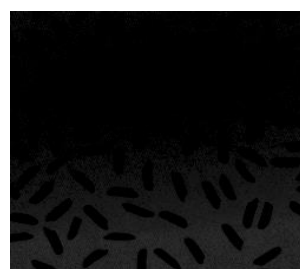
Figure 9. Approximated non-uniform background image extraction using histogram equalization
