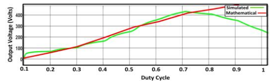
Fig. 5 Comparison of output voltage variation with varying duty cycle of the CCBC with simulated and mathematical analysis.
