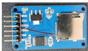
Fig. 8. SD-card adapter after modification.
