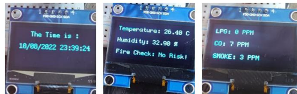
Fig. 14. OLED display on the receiver side for all parameters.
