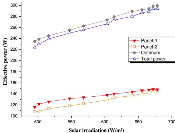
Fig. 10. The experimental and optimal power production of the PV system.
