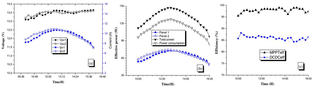
Fig. 14. Typical experimental results of the PV system operation: (a) Voltage and current (b) power production and consumption (c) Efficiency of MPPT control and DC/DC converters.
