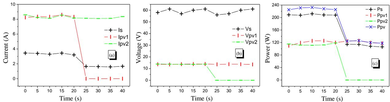
Fig. 13. Electrical values of the PV system in the presence of a fault at PVG-2: (a) current, (b) voltage and (c) power.
