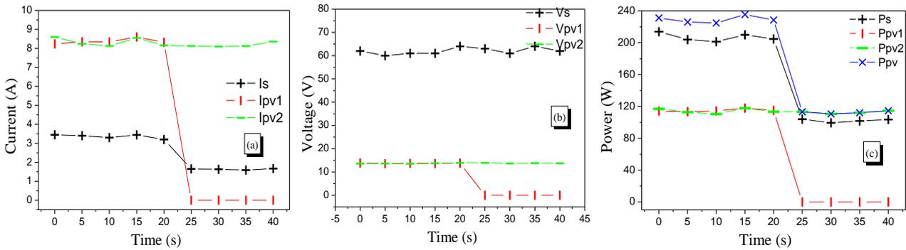
Fig. 12. Electrical values of the PV system in the presence of a default at the DC/DC1 converter: (a) current, (b) voltage and (c) power.
