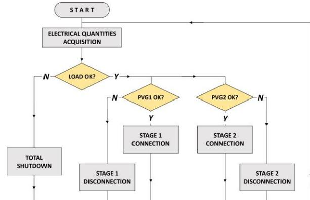
Fig. 7. The functional flowchart of the protection block.
