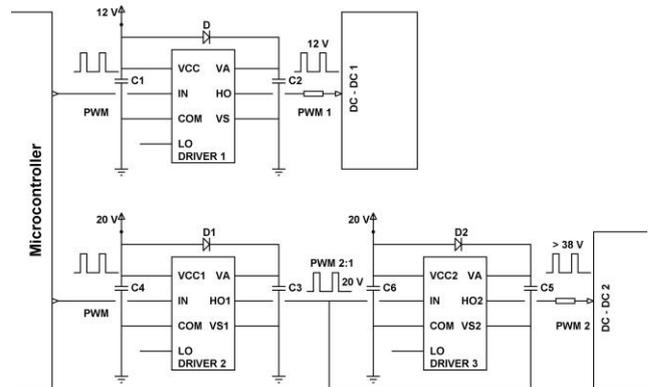
Fig. 5. Electrical diagram of the driver-based control block.
