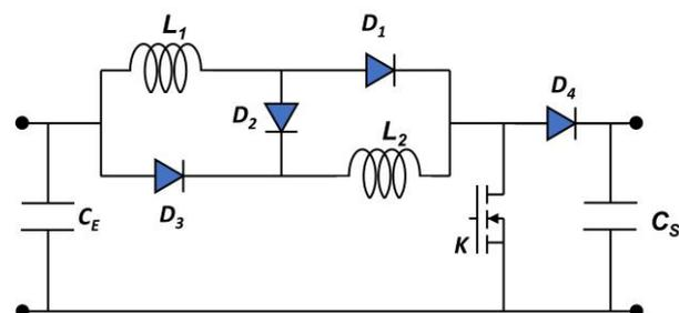
Fig. 3. Electrical diagram of the Boost DC-DC converter.
