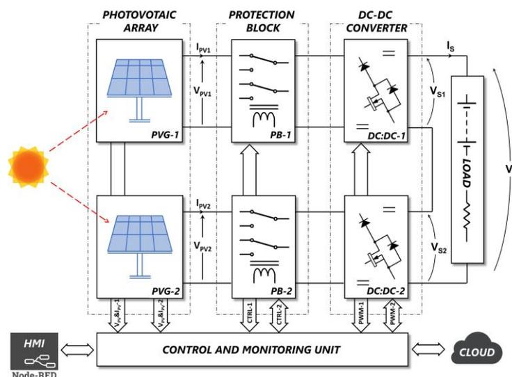
Fig. 1. Synoptic diagram of the discretized photovoltaic chain.
