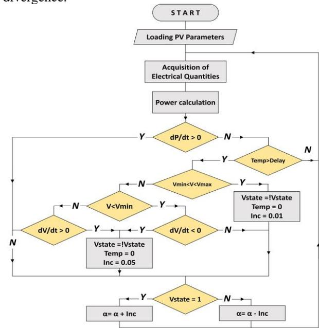
Fig. 2. MPPT algorithm implemented in the microcontroller to drive the PV system.
