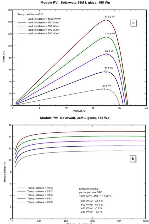
Fig. 4. (a) Experimental characteristics of the electrical power and voltage of the Module 36M L-glass 155 [32]. (b) PV panel efficiency as a function of temperature and illumination.
