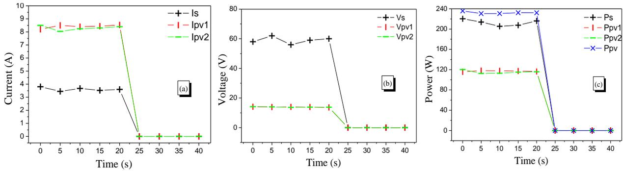
Fig. 11. Electrical values of the PV system in the presence of a load default: (a) current, (b) voltage and (c) power.
