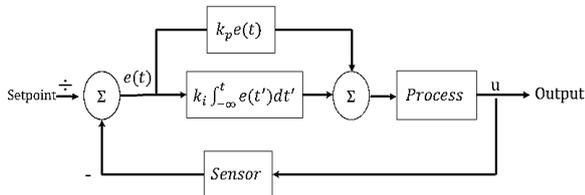
Fig. 3. Typical PI controller structure for process control
