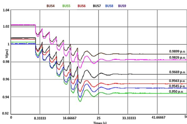
Fig. 10. Voltage recovery of all buses due to PV penetration.
