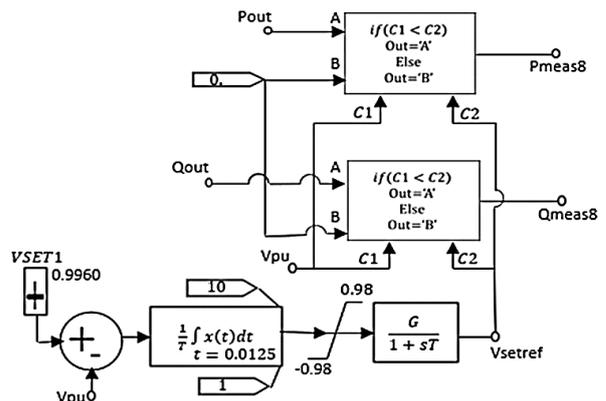
Fig. 5. PID controller design in RTDS.
