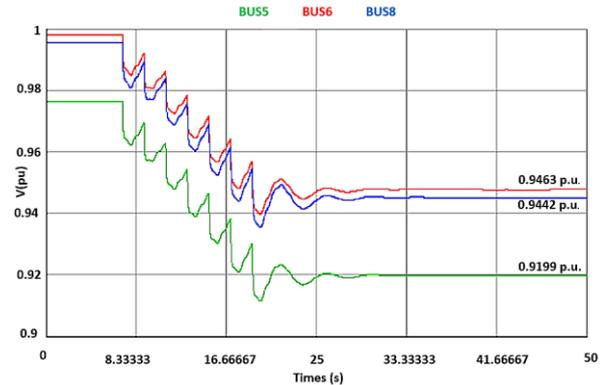
Fig. 7. Voltage drops at buses 5,6 and 8 due to a 35% increase in load consumption.
