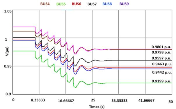
Fig. 8. Overview of the voltage drop of the entire system after disturbance.
