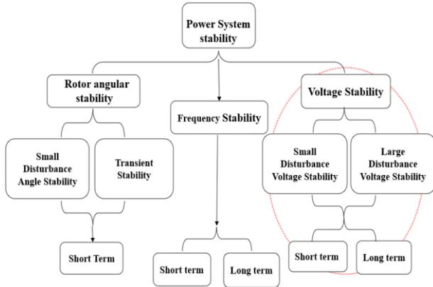
Fig. 1. Classification of power system stability according to the IEEE/CIGRE joint task force on stability terms and definition.
