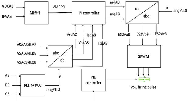
Fig. 2. Modified block design of the proposed controller for PV integration into the transmission power system.
