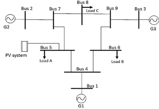
Fig. 6. IEEE 9 bus grid-tied system for simulation in RTDS.
