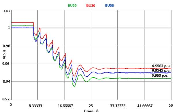
Fig. 9. Bus 5, 6 and 8 voltage response due to PV integration.
