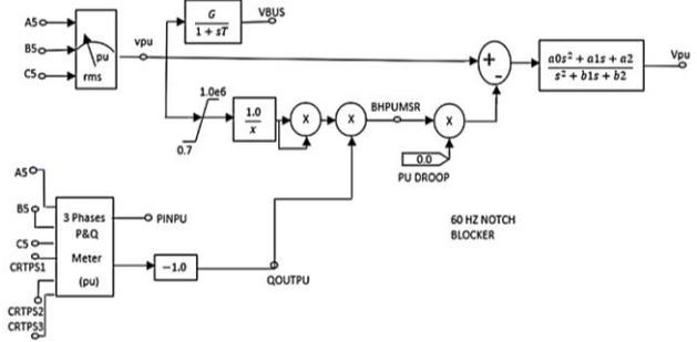
Fig. 4. Logic control for voltage monitoring at point of common coupling in RTDS.
