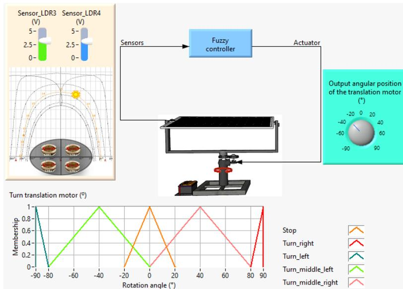
Fig. 7. Interface of the response of Motor2 related to the translation of the Earth.
