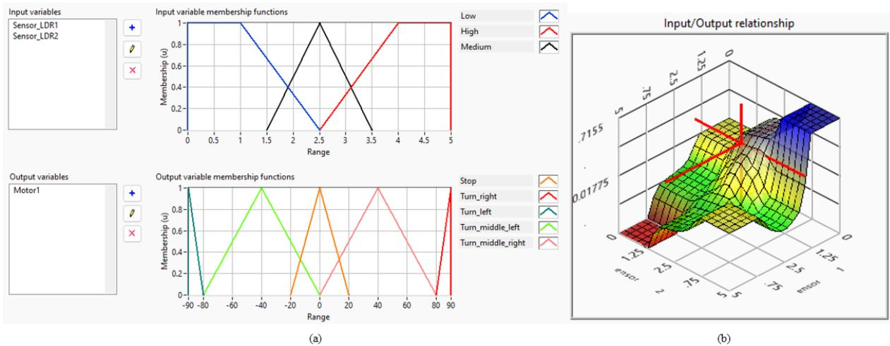
Fig. 4. (a) Input/output variable membership functions and (b) input/output relationship; for control of rotation Motor1
