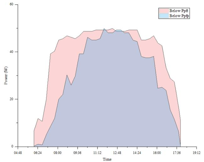
Fig. 8. Solar efficiency ratio between PV panel with solar tracker ( $P_{pft}$ ) and fixed position PV ( $P_{pfp}$ ) on a clear day.
