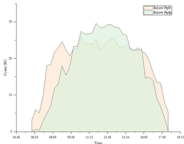
Fig. 9. Solar efficiency ratio between PV panel with solar tracker ( $P_{pft}$ ) and fixed position PV ( $P_{pfp}$ ) on a cloudy day.
