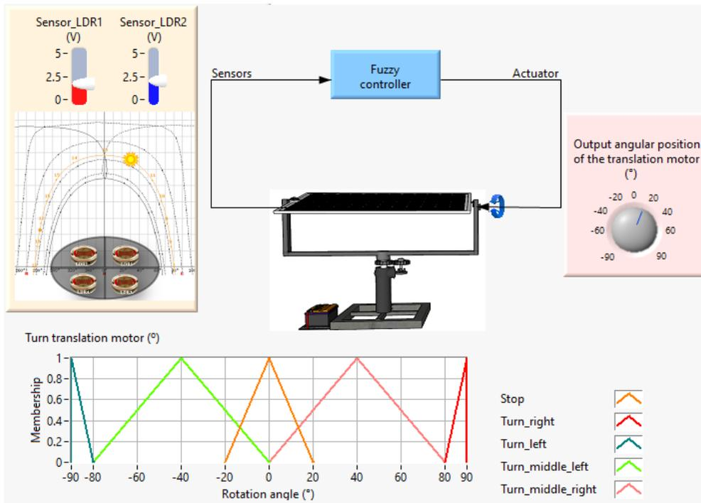
Fig. 5. Interface of the response of Motor1 related to the rotation of the Earth
