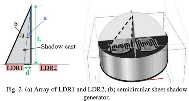
Fig. 2. (a) Array of LDR1 and LDR2, (b) semicircular sheet shadow generator.
