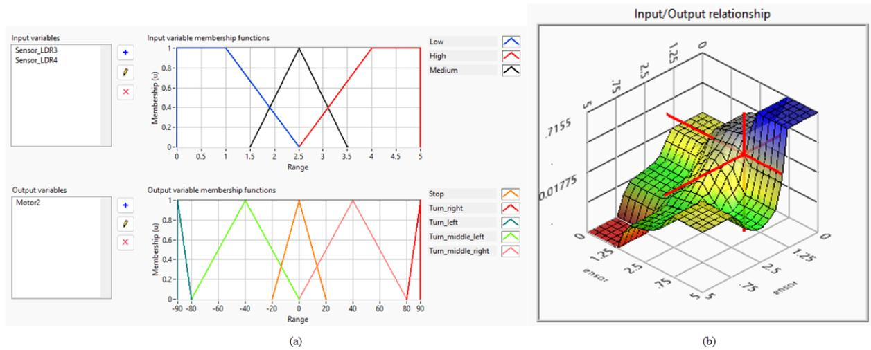
Fig. 6. (a) Input/output variable membership functions, (b) input/output relationship for translation Motor2 control.
