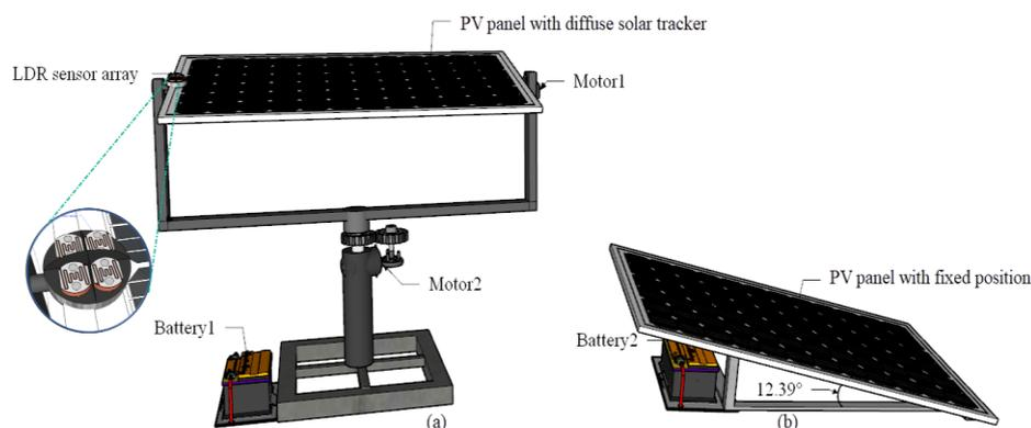
Fig. 1. (a) Structure of the proposed solar tracker and (b) photovoltaic panel with fixed position.
