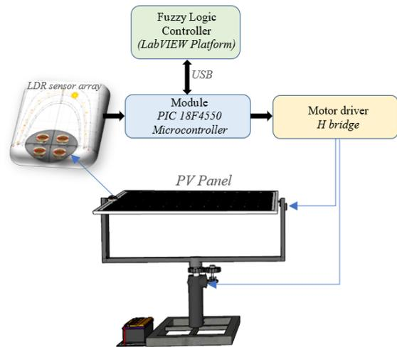
Fig. 3. Block diagram of the solar tracker with fuzzy controller.
