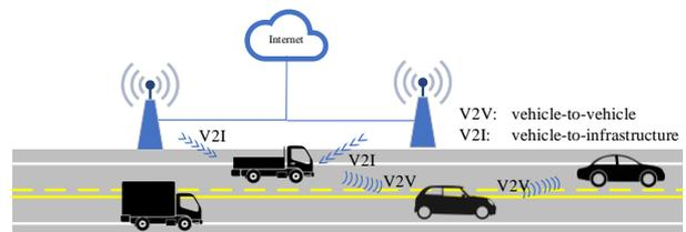
Fig. 1. The applications of DSRC technology in Vehicle-to-Vehicle (V2V) and Vehicle-to-Infrastructure (V2I) communications.
