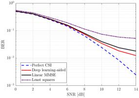
Fig. 5. BER versus the SNR [dB] with the Doppler frequency 30 Hz.
