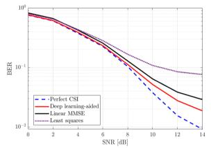
Fig. 6. BER versus the SNR [dB] with the Doppler frequency 50 Hz.
