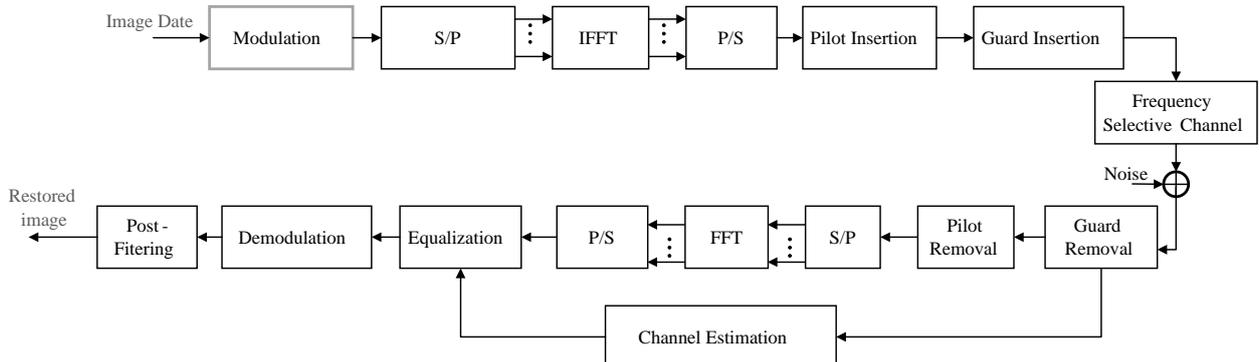
Fig. 2. The considered OFDM-based DSRC communication system over the frequency selective channels.
