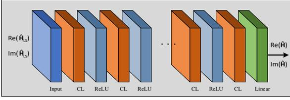
Fig. 4. The considered CNN architecture to learn and predict frequency-selective channels.
