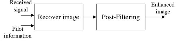
Fig. 3 The proposed receiver architecture comprising two main activities: Recover image based on the received signal and pilot information; Exploit a filter to remove noise and artifacts.
