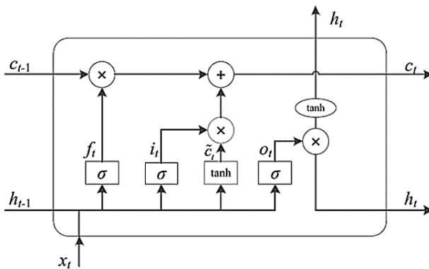
Fig. 2. LSTM structure network.
