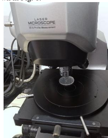
Fig. 1. 3D laser microscope measurement of epoxy resin replica.
