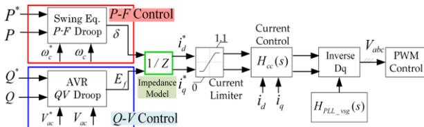
Fig. 4. Control schemes of the VSG control.
