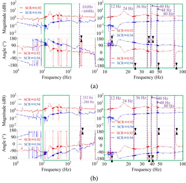
Fig. 11. Bode plots of the eigenvalues SISO minor-loop gain: (a) Bode plots of  $\lambda_p$  (The right is an enlargement of the left) and (b) Bode plots of  $\lambda_n$  (The right is an enlargement of the left).
