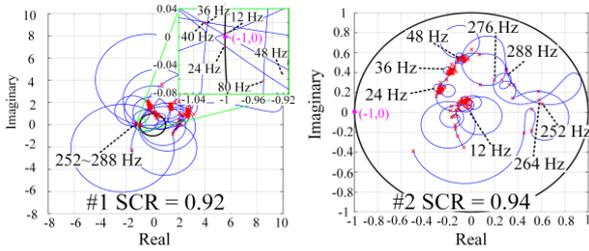
Fig. 12. Eigenvalue loci of the SISO minor-loop gain.
