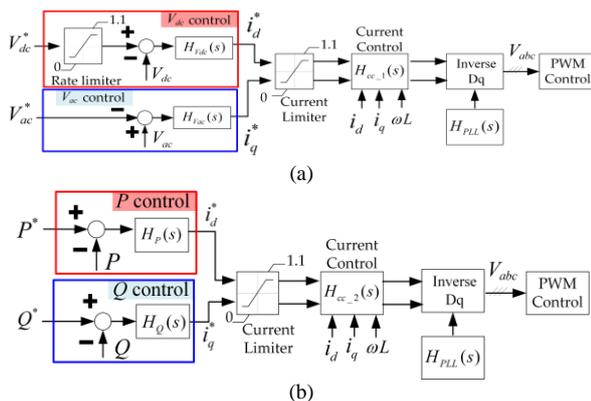
Fig. 2. Control schemes of MMCs: (a) Voltage control scheme of MMC<sub>1</sub> and (b) Power control scheme of MMC<sub>2</sub> (Conventional PQ control).
