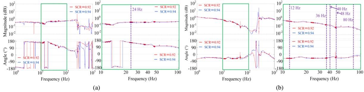
Fig. 14. Bode plots of the eigenvalues of the dq MIMO minor-loop gain, using the VSG control for MMC<sub>2</sub> in T2: (a) Bode plots of  $\lambda_1$  (The right is an enlargement of the left) and (b) Bode plots of  $\lambda_2$  (The right is an enlargement of the left).
