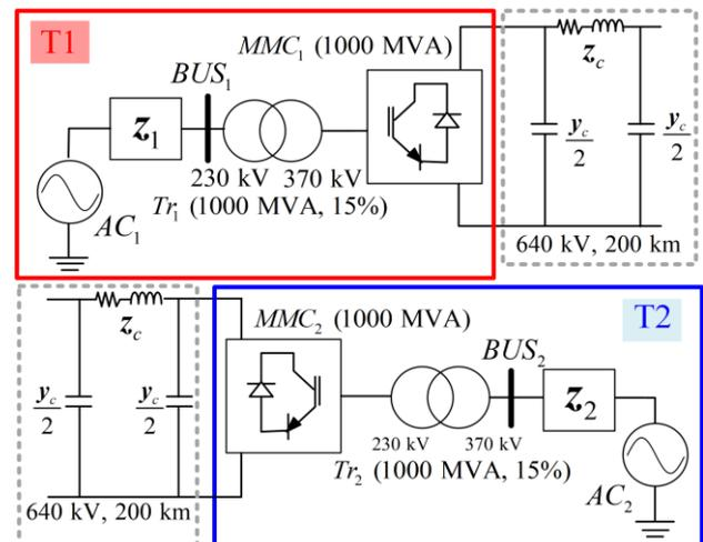
Fig. 1. Topology of a symmetrical monopolar HVDC.
