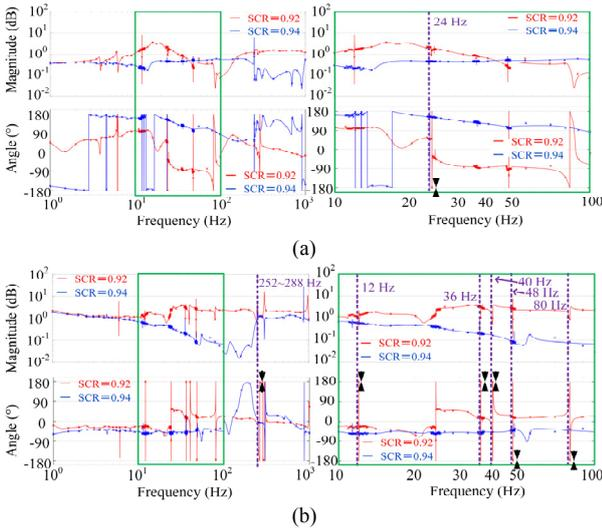
Fig. 8. Bode plots of the eigenvalues of the MIMO minor-loop gain: (a) Bode plots of  $\lambda_1$  (the right is an enlargement of the left) and (b) Bode plots of  $\lambda_2$  (the right is an enlargement of the left).
