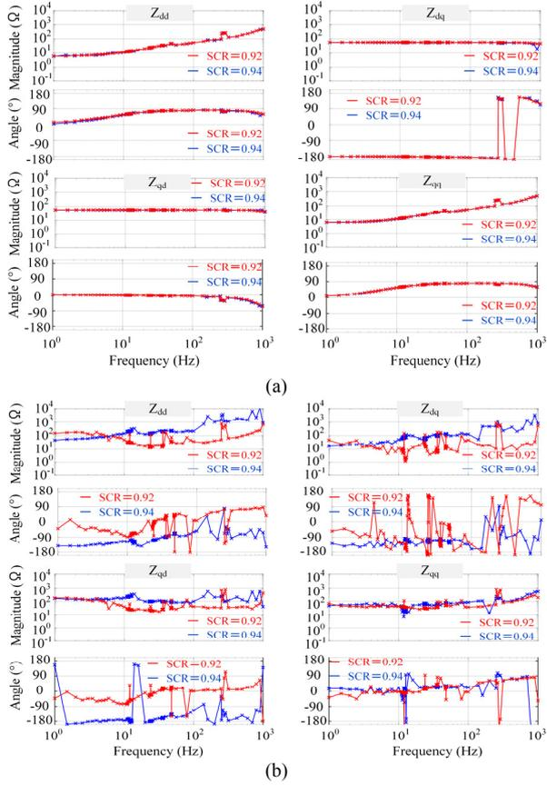
Fig. 7. dq MIMO impedances of sub-circuits: (a) Output impedance of source-side ( $Z_s^{dq}(s)$ ) and (b) Output impedance of load-side ( $Z_L^{dq}(s)$ ).
