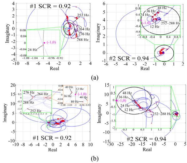
Fig. 9. Nyquist plots of the eigenvalues of the MIMO minor-loop gain: (a) Eigenvalue loci of  $\lambda_1$  and (b) Eigenvalue loci of  $\lambda_2$ .
