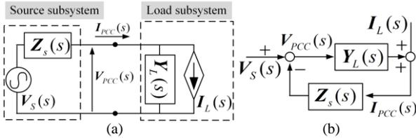
Fig. 6. Splitting of the general power system into source and load subsystems represented by Thévenin and Norton equivalents: (a) Thévenin and Norton equivalents and (b) Block diagram of the equivalent circuit.
