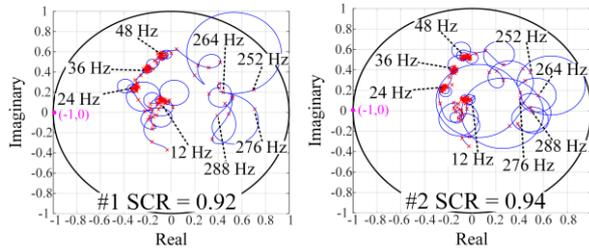
Fig. 18. Eigenvalue loci from the minor-loop gain derived from the SIO impedance, using the VSG control for  $MMC_2$  in T2.
