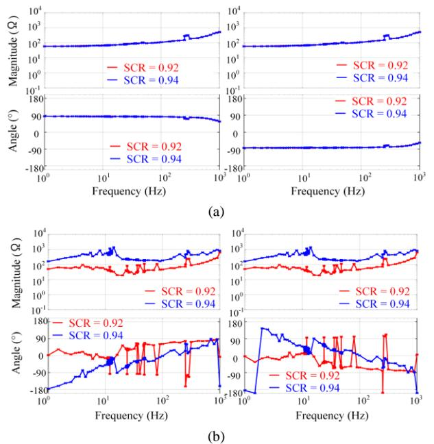
Fig. 10. Equivalent SISO impedance of sub-circuits: (a) Source-side impedance ( $Z_s^{pn}$ ) and (b) Load-side impedance ( $Z_L^{pn}$ ).
