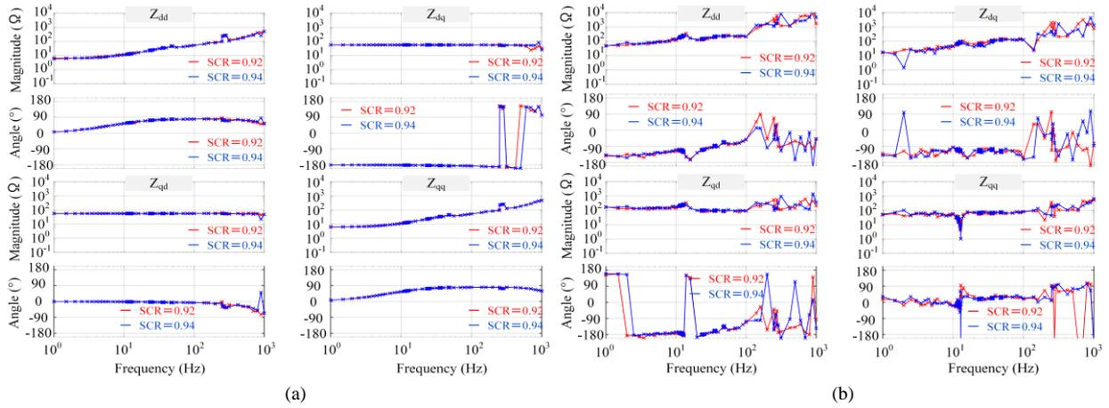
Fig. 13. dq MIMO impedances of the sub-circuits, using the VSG control for MMC<sub>2</sub> in T2: (a) Output impedance of source-side ( $Z_s^{dq}(s)$ ) and Output impedance of load-side ( $Z_L^{dq}(s)$ ).
