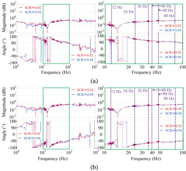
Fig. 17. Bode plots of the eigenvalues SISO minor-loop gain, using the VSG control for  $MMC_2$  in T2: (a) Bode plots of  $\lambda_p$  (the right is an enlargement of the left) and (b) Bode plots of  $\lambda_n$  (the right is an enlargement of the left).
