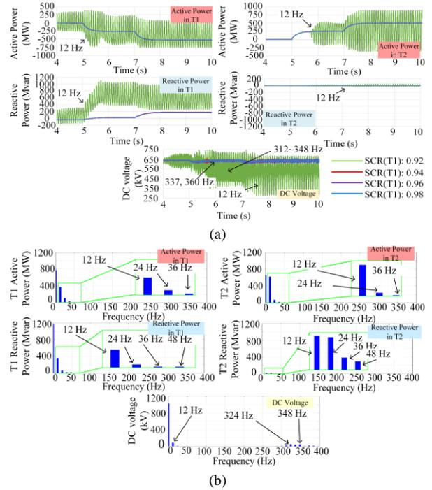
Fig. 3. Time responses and discrete Fourier transform results with Conventional PQ control: (a) Time response of active/reactive powers and DC voltage and (b) Discrete Fourier transform (DFT) applied to time responses.
