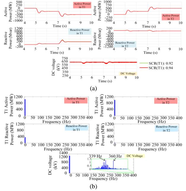
Fig. 5. Time responses and discrete Fourier transform results with VSG power control: (a) Time responses with VSG power control and (b) DFT applied to time responses.
