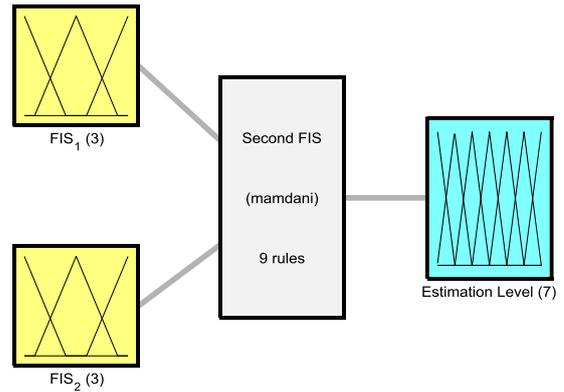
System Second FIS: 2 inputs, 1 outputs, 9 rules
