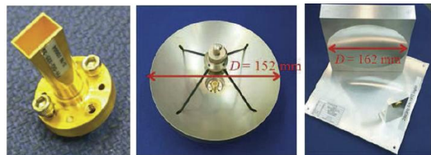
Fig. 8. Rectangular horn, cassegrain, and parabolic antennas, respectively [96].
